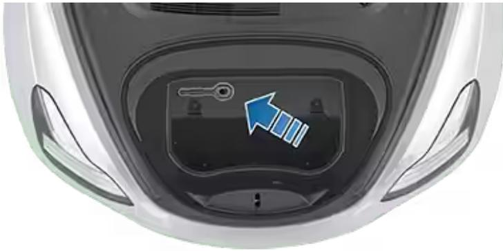
2. Release the tow eye cover by pressing firmly on its top right perimeter until it pivots inward, then gently pulling the raised section toward you.
