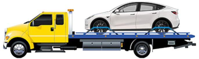
If Model Y must be transported without a flatbed truck, then wheel lifts and dollies must be used to ensure that all four wheels are off of the ground. This method may only be used for a maximum of 35 miles (55 km), and must not exceed the manufacturer speed rating of the dollies. With this method, Tesla recommends the vehicle facing forward so that the front wheels are lifted and the rear wheels are on dollies.
