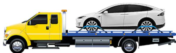
If Model X must be transported without a flatbed truck, then wheel lifts and dollies must be used to ensure that all four wheels are off the ground. This method may only be used for a maximum of 35 miles (55 km), and must not exceed the manufacturer speed rating of the dollies. With this method, Tesla recommends the vehicle facing forward so that the front wheels are lifted and the rear wheels are on dollies.
